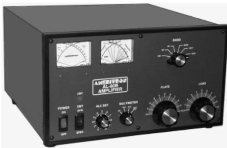
Ameritron's AL-80B kilowatt *output* desktop linear can double your average SSB power output with high-level RF processing using Ameritron's exclusive *Dynamic ALC*<sup>TM</sup>.
